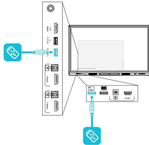
The following table shows which USB Type-A receptacles you can use with each input source and the supported USB speed:
