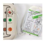
Stick pads to casualty as illustrated on the pads. The visual indicator on the device will also light up to illustrate where to stick the pads.
